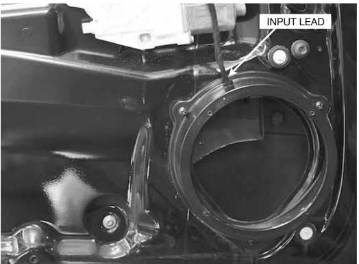
Before you assemble the woofer-midrange on the adapter ring, it must be connected (connector enclosed!) with the original speaker cable.
