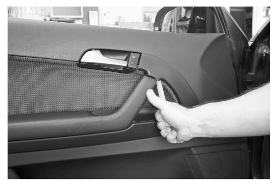
Prize away the door covering with a plastic wedge. Work bottom-up. After that, slide the cover panel upwards out of the window seal.
